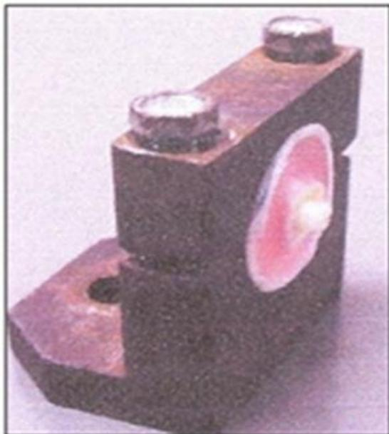
**Figure 5.** Samples were positioned on the shear guillotine
