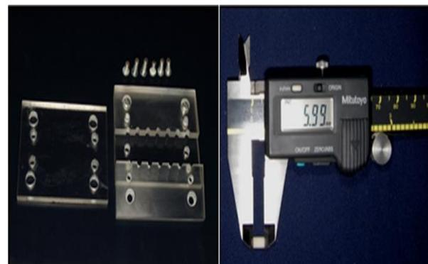
**Figure 1.** Teflon split mould and micrometer screw gauge (Kawasaki, Japan)
