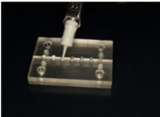
**Figure 2.** The nozzle of the capsule was inserted into the cavity of the mould and touched to the wall of the mould
