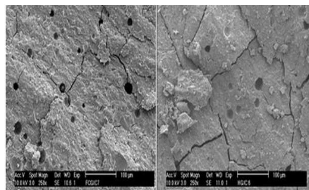
**Figure 3B.** Scanning electron microscopy photomicrograph showing the porosity at the fracture surface of Fuji I CAPSULE
