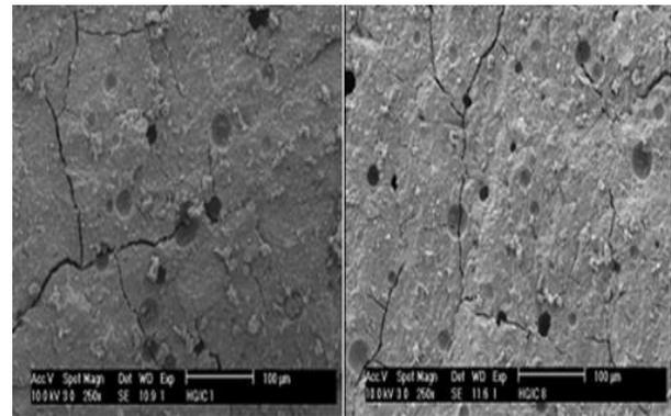
**Figure 3A.** Scanning electron microscopy photomicrograph showing the porosity at the fracture surface of Fuji I
